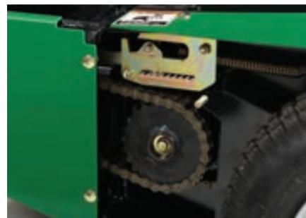
Automatic tensioning on the main drive chains ensure proper tension during operation and reduces required maintenance.
