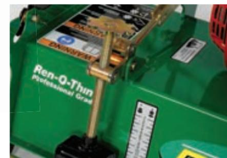
Infinite height adjustment allows you to change the height of the deck to obtain the best performance.
