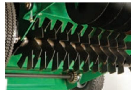
Durable cutting blades can be adjusted down to a depth of 1½".
