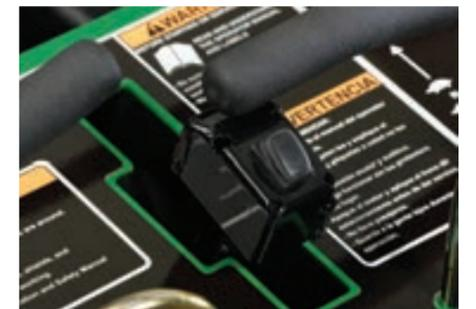
Tine lift switch to raise and lower tines conveniently located near control lever.
