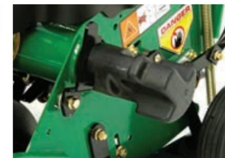
Removable weights lighten the load for easier lifting and transporting.
