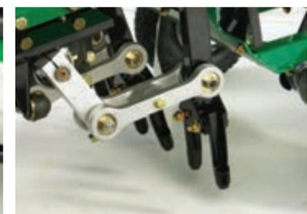
Reciprocating tines provide vertical coring action, punching straight in and out without tearing the turf, offering golf course quality results.
