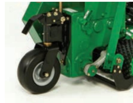
Pneumatic swiveling rear wheel makes it easy to maneuver tightly around turns and cut closely along contoured landscape edges.
