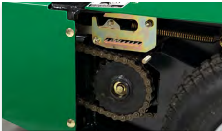
Innovative automatic chain tensoning system reduces the chain maintenance required
