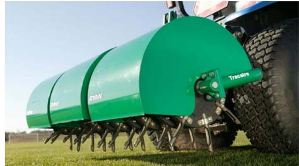
*Tracaire Aerator above (shown topless below) alleviates compaction in high traffic flat areas.*
