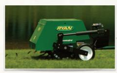
For maximized productivity, independently mounted tine wheels let you make turns while the tines are in the ground.
