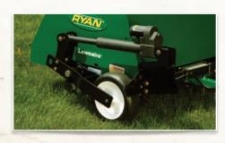
A variety of available lifting mechanisms allow you to easily lift and lower your aerating unit.
