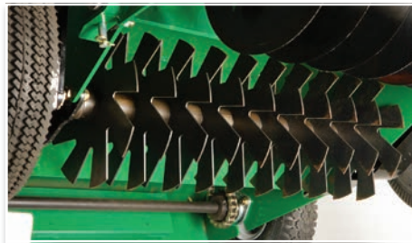
Durable cutting blades can be adjusted down to a depth of 1 1/2".
