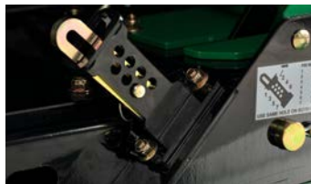
Aeration and consistent coring depth control for precision aeration in varying soil conditions; aerates up to 5" deep, in half-inch increments.
