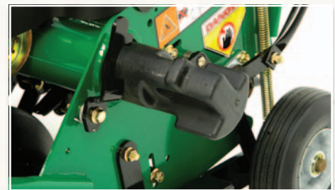
Weights are easily and conveniently removable for easier lifting and quicker, less strenuous transportation.
